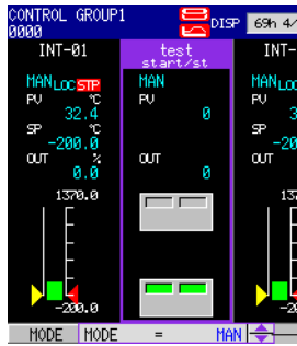
Auto/manual switching window
